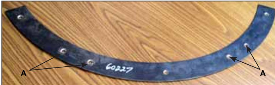
6. Countersink the holes in the casting that correspond with the holes labeled “A” in Figure 2 to 3/8 in. x 82° and blow out the holes with compressed air.
