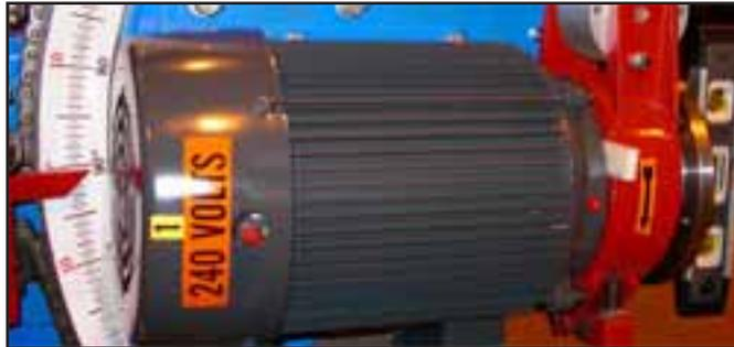
11. If a scale must be adjusted, turn off and lockout/tagout all power to the saw. Repeat steps 8 and 9 until each angle scale label is in the proper position.
